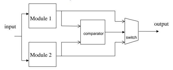
Sometimes named dual-modular redundancy
