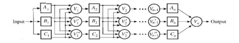
The effect of partitioning of modules (A, B, C) is that the design can withstand more failures than the solution with only one large triplicated module
