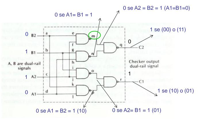
Set of faults: stuck-at-1, stuck-at-0 of each line (a, b, c, d, e, ...., q, r)
