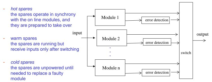
Reconfiguration process can be viewed as a switch that accepts the module's outputs and *error reports* As long as the outputs agree, the spares are not used. When a miscompare occurs, the switch uses the error reports from the modules to identify the faulty module and then select a replacement module.
