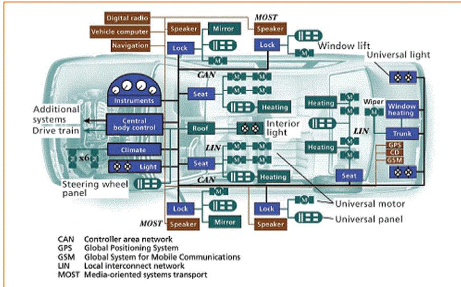
Over 80 different embedded processors, interconnected with each other.
