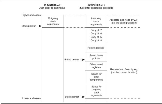
Figure 7–3. Stack Frame Using Variable Arguments
