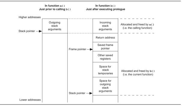
Each section of the current frame is aligned to a 32-bit boundary. The ABI requires the stack pointer be 32-bit aligned at all times.
