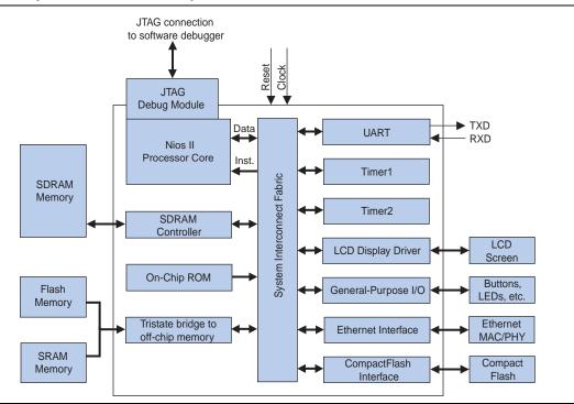
If the prototype system adequately meets design requirements using an Altera-provided reference design, you can copy the reference design and use it without modification in the final hardware platform. Otherwise, you can customize the Nios II processor system until it meets cost or performance requirements.
