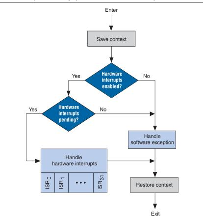
Figure 8–1. HAL Exception Handling System with the Internal Interrupt Controller
