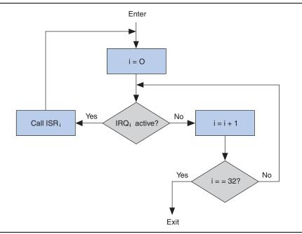
Figure 8–2. HAL Hardware Interrupt Funnel for the Internal Interrupt Controller
