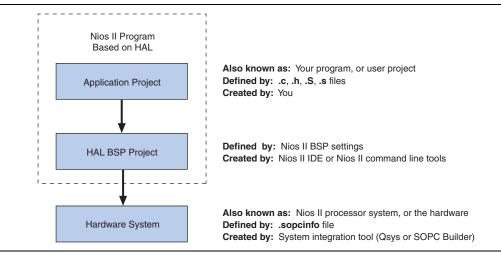
Every HAL-based Nios II program consists of two Nios II projects, as shown in Figure 6–1. Your application-specific code is contained in one project (the user application project), and it depends on a separate BSP project (the HAL BSP).
