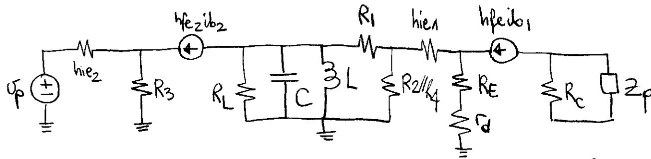
$$Z_p = h_{ie2} + R_3(h_{fe2} + 1) = 204.2 \quad | Z_L = R_L \parallel \frac{1}{C_s} \parallel L_S = \frac{R_L L_S}{R_L C_s^2 + L_S + R_L}$$
