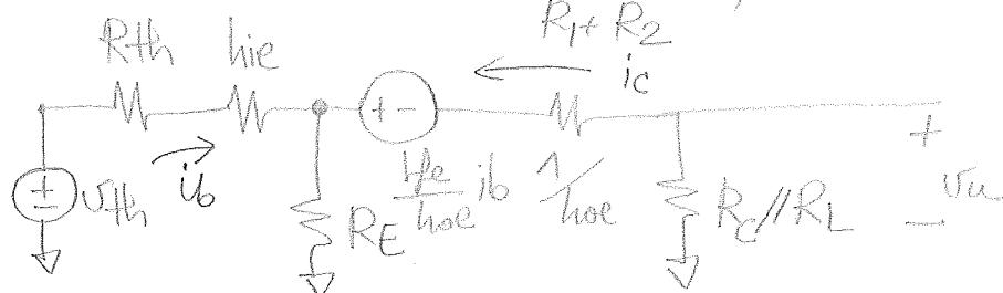
$$\left\{ \begin{array}{l} V_{Th} = (R_{Th} + h_{oe})i_b + R_E(i_b + i_c) \end{array} \right.$$
