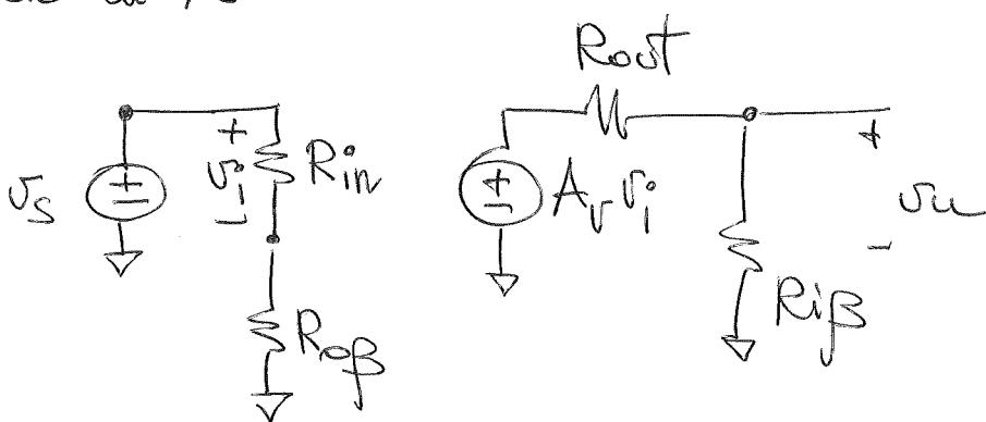
$$A_e = \frac{R_{if}}{R_{if} + R_{out}} \quad A_v = \frac{R_{in}}{R_{in} + R_{of}}$$
