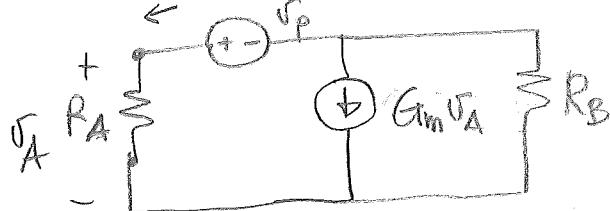
$$R_A = (R_1 // R_2 + r_{bb}') // (r_{be}' + R_E (1 + g_m r_{be})) = 2139 \Omega$$
