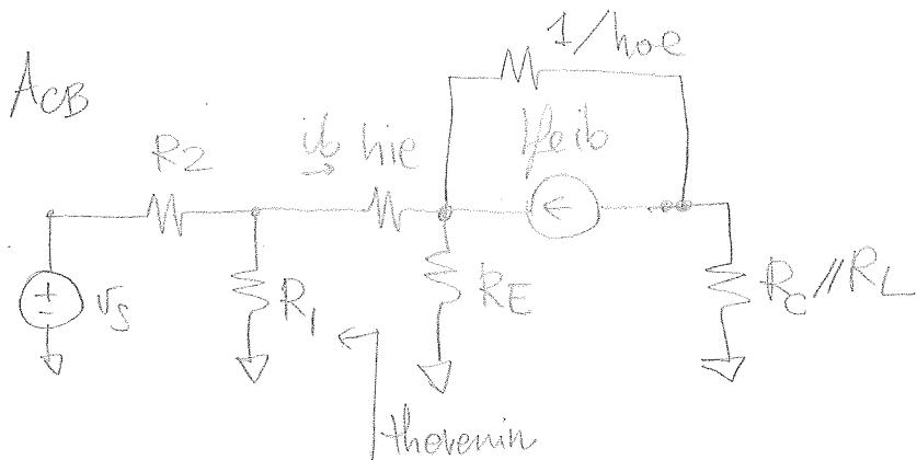
$$V_{Th} = \frac{V_S R_1}{R_1 + R_2}, \quad R_{Th} = R_1 // R_2$$
