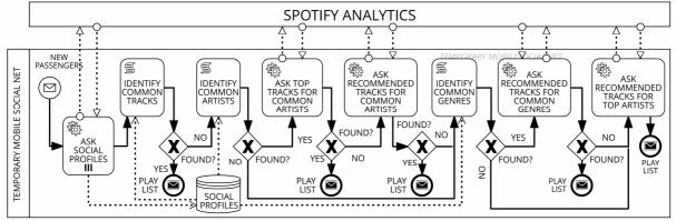
Figure 5 BPMN protocol of an audio streaming recommender based on TMSN and Spotify analytics.
