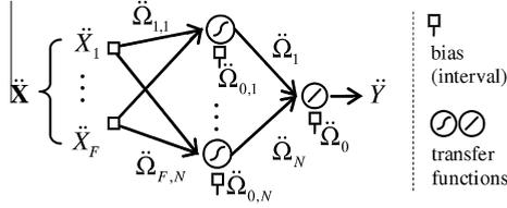
Fig. 2. The proposed MLP architecture for interval-valued data.
