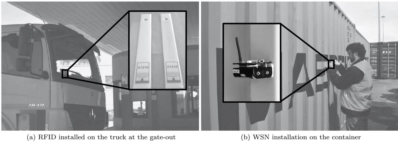
(a) RFID installed on the truck at the gate-out
