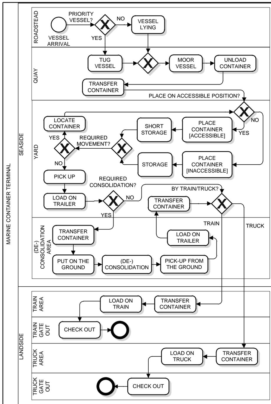
Fig. 3: BPMN model of a container terminal system.
