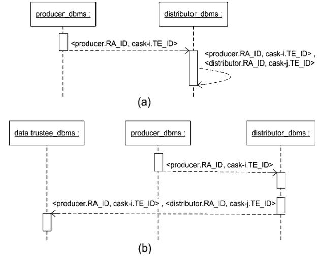
**Figure 4. Sequence diagram of a purchase activity; (a) distributed architecture (b) centralized architecture.**
