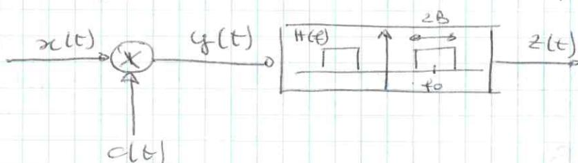
$$\text{con } c(t) = \sum_{m=-\infty}^{+\infty} c_0(t-mT), \quad c_0(t) = \delta(t) - \delta(t - \frac{T}{2}), \quad T = 4/B, \quad f_0 = 2B.$$
