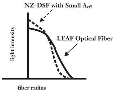
LEAF fiber's larger  $A_{eff}$  increases the area where the light can propagate, thereby reducing non-linear effects.
