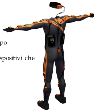
Fig. 1. Xsens MVN consists of 17 inertial and magnetic sensor modules. Data is transmitted by a wireless connection to the laptop computer on which the processing is performed and visualized. A suit is used for quick and convenient placement of sensors and cables.
