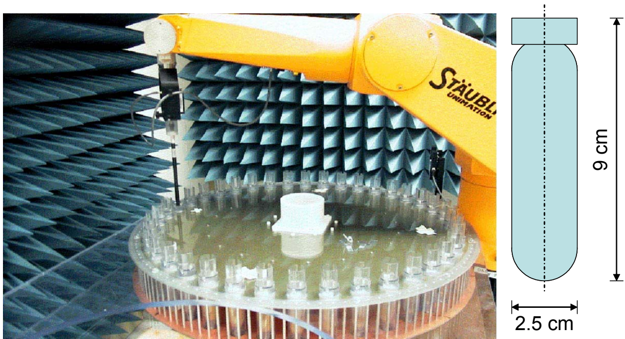
Fig. 5. SAR measurements along the dummy load centerline by means of a miniature E-field probe.
