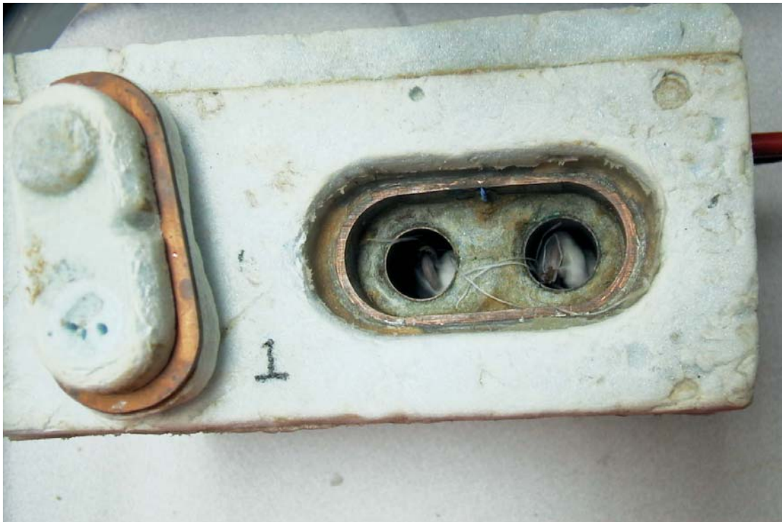
Fig. 4. Twin-well calorimeter loaded with exposed and sham-exposed 23-gram mice.
