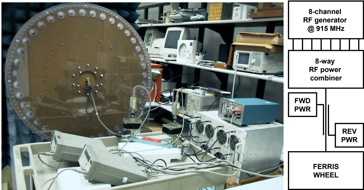
Fig. 2. RF power generation and monitoring setup.
