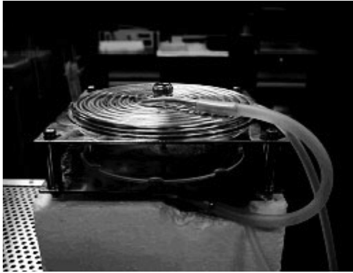
Fig. 3. Wire patch cell operating at 1800 MHz with four Petri dishes and a thermostated water jacket as reported in [45, Fig. 11].
