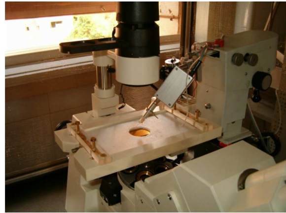
Fig. 4. CPW system for patch-clamp recordings while mounted on a microscope, as used in the laboratory of the Department of Human and General Physiology, University of Bologna.
